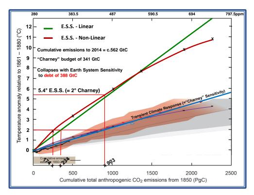
However, when we apply the full Earth System Sensitivity, the equilibrium planetary response to anthropogenic emissions can be seen to have exceeded the policy target (of a maximum increase of  $2^{\circ}$ C) as the cumulative emissions passed 174 GtC.
