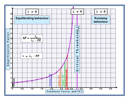
The non-linear relationship between Amplification Factor and Feedback Factor is immediately obvious. AF depends on the difference between  $\lambda_0$  and the FF. AF approaches infinity as the gap approaches zero.
